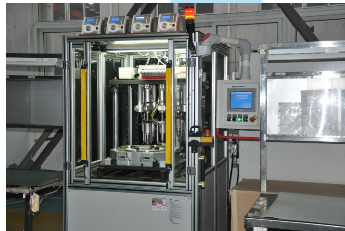
热熔焊接 Hot Melt Welding
